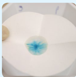
Fig.1 Sample of Cobalt Thiocyanate Color Test
